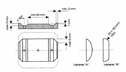
Since 1995 only cleat plates according to the above draft have been used. The equipment check can be done directly after the run. The use of non-homologated elements, may lead to disqualification.
